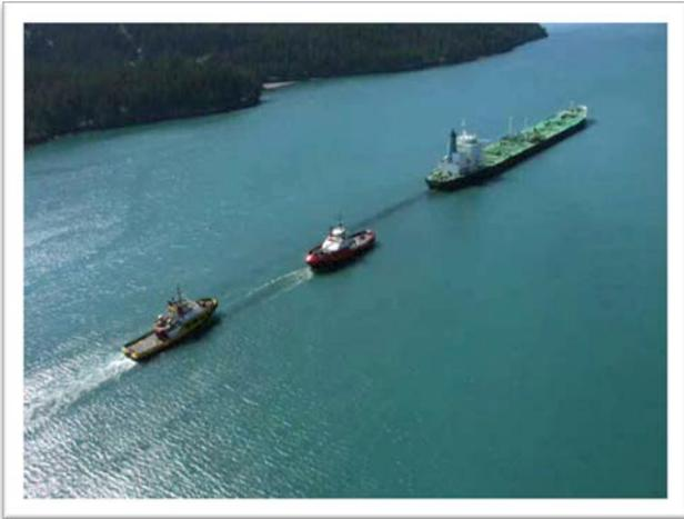
*Figure 3.3 Laden tanker in Prince William Sound being escorted by two tugs (PWSRCAC photo)*
