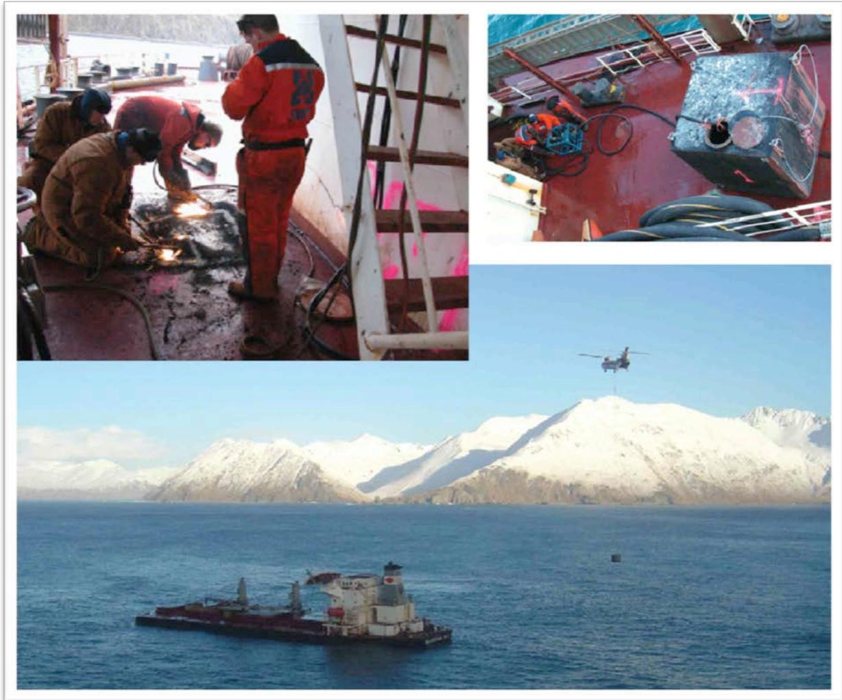
*Figure 3.5 Salvage operations on the M/V Selendang Ayu in the Aleutian Islands included lightering the remaining fuel from the vessel. Holes were drilled in the deck so that fuel oil could be pumped into containers that were then airlifted by a heavy-lift helicopter from the remaining portion of the vessel hull to land. (Unified Command photos)*
